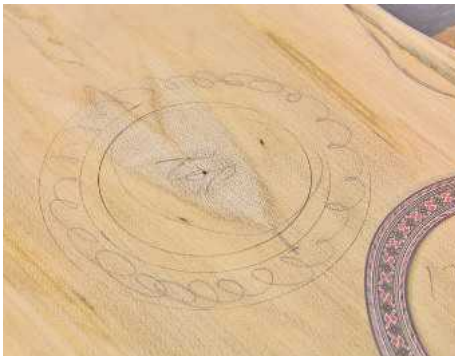
▲ Pic.4 The inner and outer lines for the rosette were cut and the sound hole lightly scored; waste was marked out
